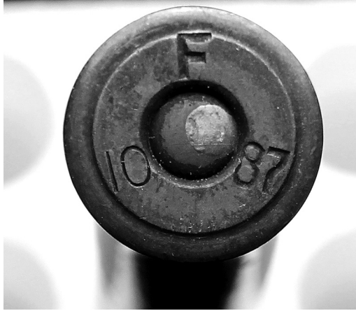
Figure 3.1 A .45–70 Government cartridge head stamp. The “F 10 87” indicates that this cartridge was manufactured by the Frankford Arsenal in Philadelphia, PA, circa October 1887. (Image from author’s collection.)
